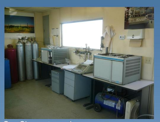
Gas Chromatographs No.1 Refinery Gas, No.2 Hydrogen and Methane
