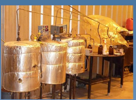
Insulated and Assembled Soak Test Units
